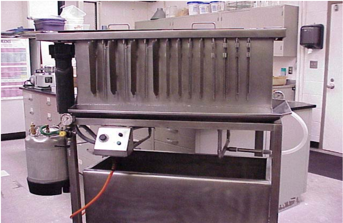
Figure 2: Picture of the spray wash cabinet used for the application of treatments onto frankfurters and Polish sausages
