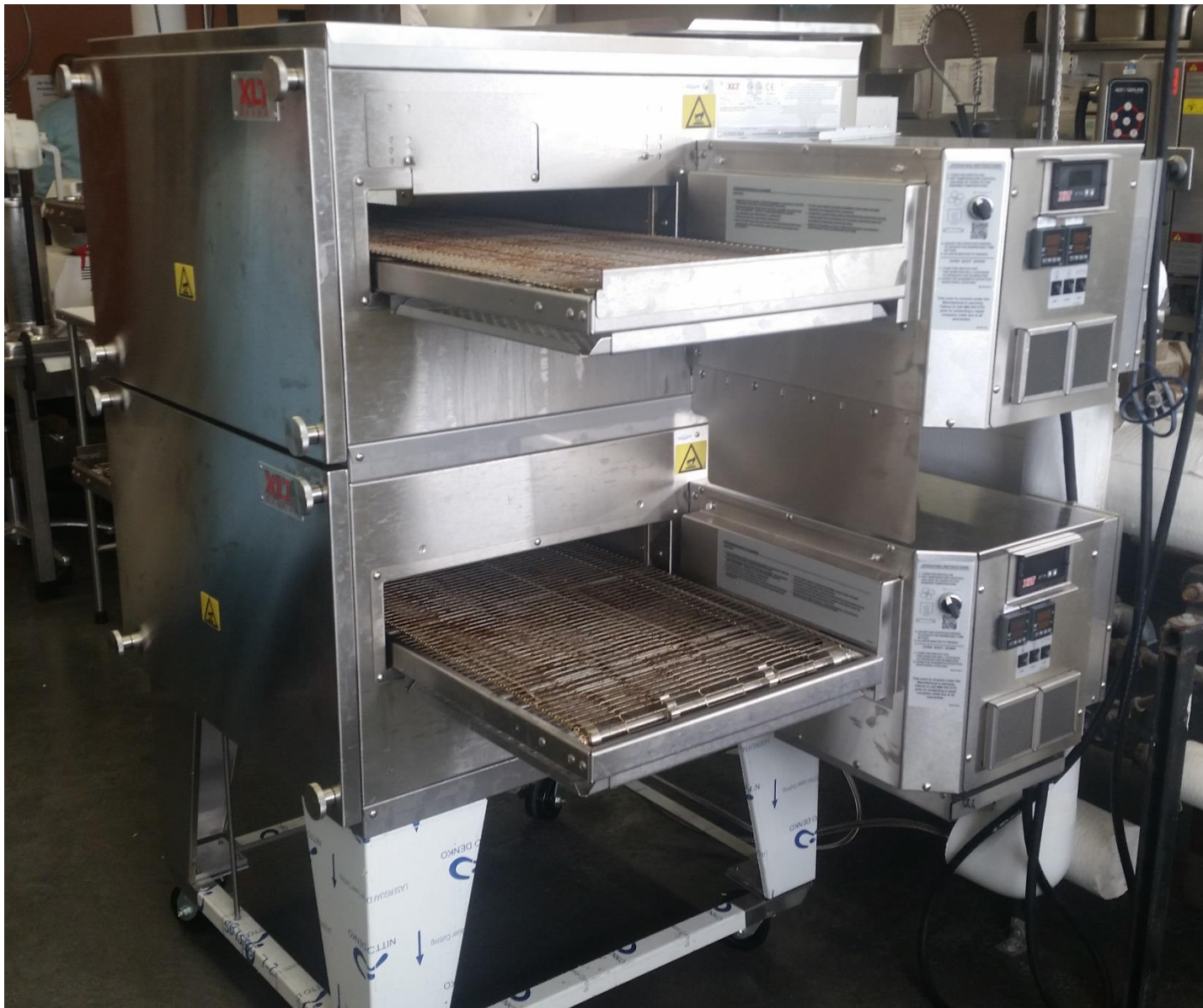
Figure 3: Physical layout of two-zone impingement ovens with relative humidity controls.
