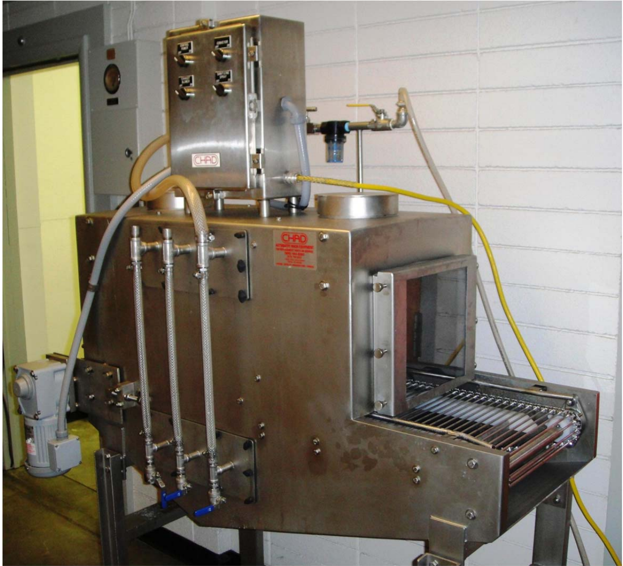
Figure 1. Custom-built spray cabinet used to apply treatments (Study 5)
