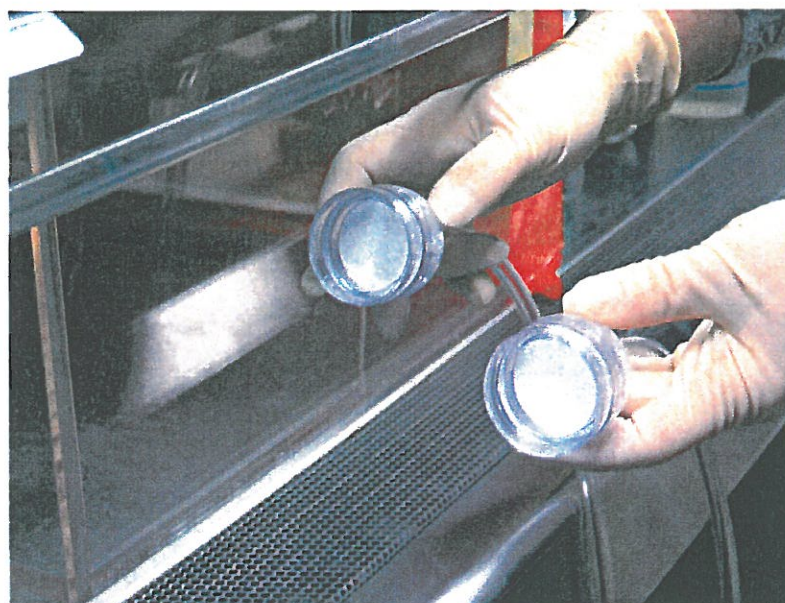
Figure 19. Shown are glass fiber filters used to trap Listeria from aerosol for analysis.
