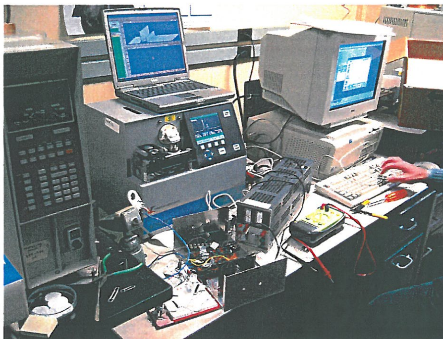
Figure 10. Final IonScan assisted by externally controlled sample heat ramp.
